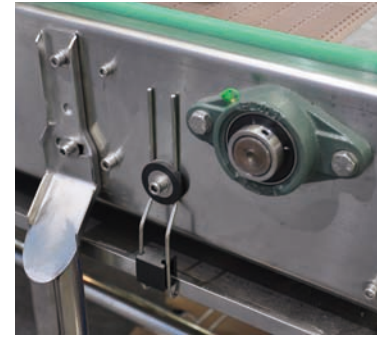
Head Of Drip Tray Supports (Material): SUS304 Washer Clamp in Polyamide
